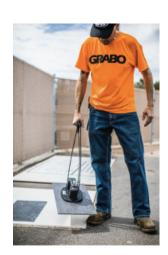
down. The actuator on the handle bar helps in controlling the functions. The Erguo S1 attachment is compatible with all models, except the Grabo H as that is designed for simpler and shorter duration usage.
